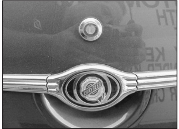
23. The Cruiser includes a lift tailgate whose lock, Strattec 705744, is separate from the handle release.
